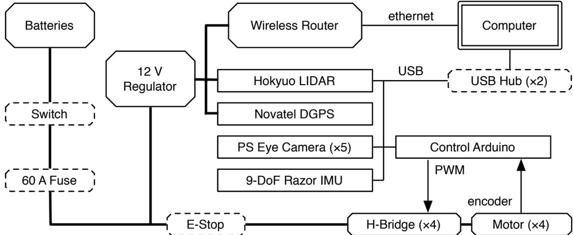
Figure 2: Electronics Diagram
