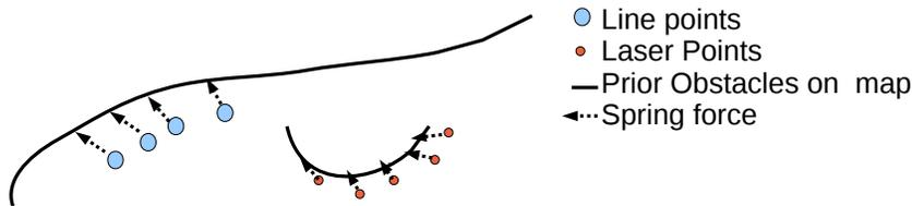
Figure 7: The Navigator uses an Iterative Closest Point (ICP) algorithm within the GMapping to align the detected line points and obstacles with the current map. At each ICP iteration, the sensor points are matched with the closest existing map obstacle with a spring (dotted arrow above). ICP aligns the data with the map to minimize total force in the springs. This minimizes the error between our prior map and current sensor data and creates a consistent world map.
